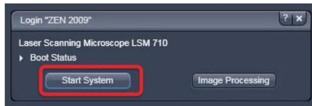
As the hardware configures, you will hear the microscope parts starting to activate. This is normal. You are now ready to image! Remember to only save files on the D: drive. **DO NOT save files on the C: drive!**
